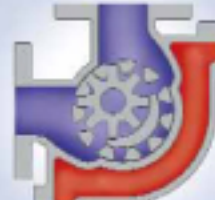
The heating jacket around the casing allows a better and constant heating of the product where it is required. In the gears. Inspections can be done with the casing connected on the pipes. For temperature-sensitive fluids it is available the heating jacket around the complete pump.
