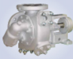
The heating jacket around the casing allows a better and constant heating of the product where it is required. In the gears. Inspections can be done with the casing connected on the pipes. For temperature-sensitive fluids it is available the heating jacket around the complete pump.
