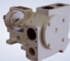
The heating jacket around the casing allows a better and constant heating of the product where it is required. In the gears. Inspections can be done with the casing connected on the pipes. For temperature-sensitive fluids it is available the heating jacket around the complete pump.
