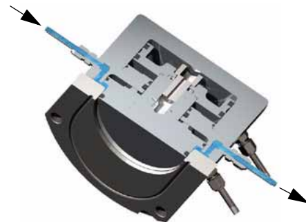
Fig. 31 Cleaning of the pressure-relief valve
