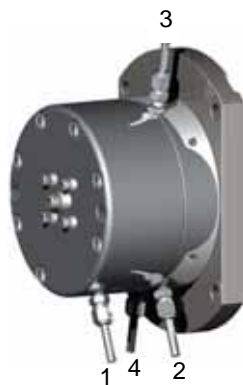
Fig. 28 Connections on pressure-relief valve
