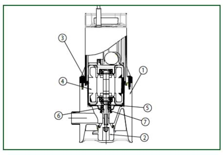
**Motor:** Two-pole asynchronous submergible type motor from 0.18 and 0.4 kW with built-in **thermal protection** and permanently connected capacitor installed in the cable compartment.
