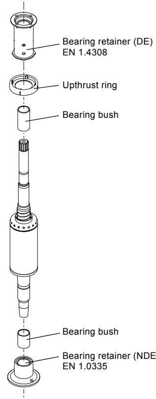
Fig. 9 Bottom and top radial bearings
