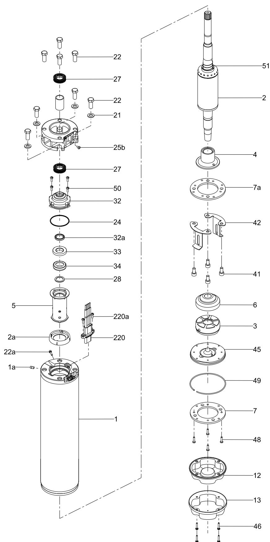
**Fig. 8** Exploded drawing of the MS6000F
