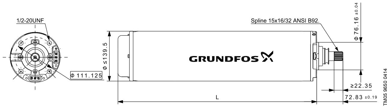
Fig. 12 Dimensional drawing of MS6000
