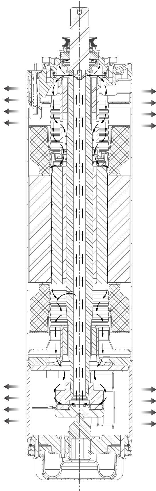
**Fig. 11** Liquid circulation inside motor
