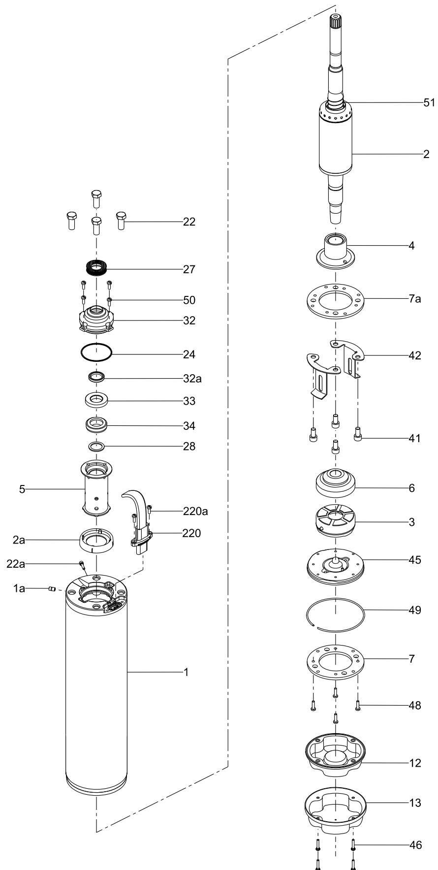
Fig. 7 Exploded drawing of the MS6000 motor
