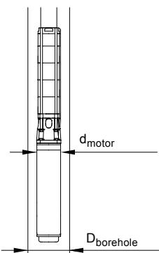
Fig. 2 Diameter of motor and borehole
