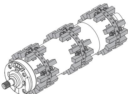
**Fig. 24** Submersible motor fitted with anode strings
