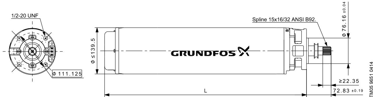
Fig. 13 Dimensional drawing of MS6000 with extension flange
