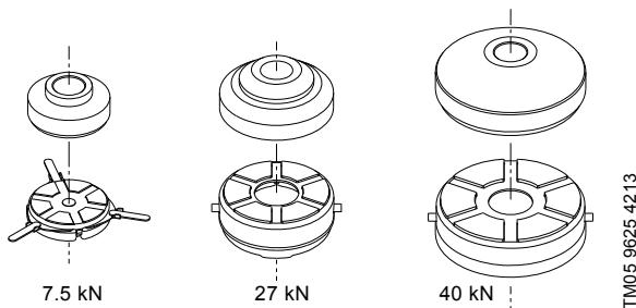
**Fig. 10** Thrust bearings
