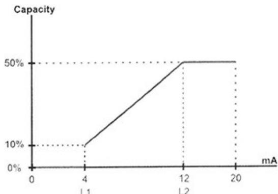
If in input there is a current of 8mA the pump performs a dosing at 30%.
