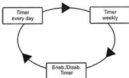
This mode allows to program the pump as a daily or weekly timer up to 7 ON/OFF operations
