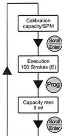
This menu allows to set the flow rate in mL of the pump in 100 strokes.
