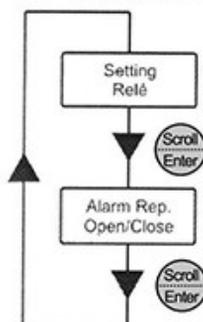
This menu allows to set the functioning of the relay output (OUT RELAY) that can be normally open or normally closed.
