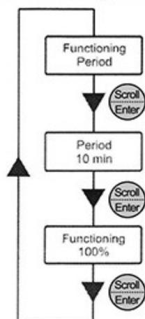
The pump doses for programmed time and flow rate.
