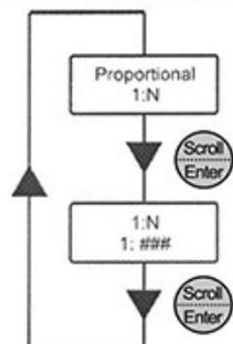
Every time that the pump receive "N" pulses from the water meter, the pump performs a stroke.
