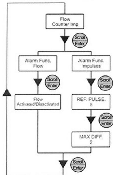
This menu allows to set the alarm function of the flow sensor. It can be:
